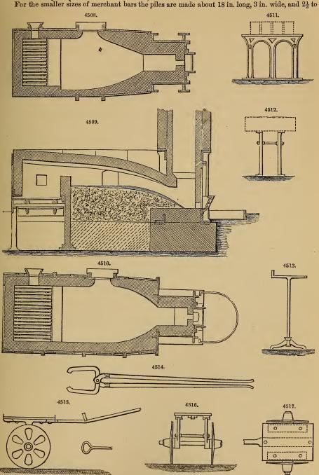
3 in. thick. The heat is composed of sixteen or eighteen piles, which take from twenty-eight to thirty minutes in reaching a welding heat. The time occupied in drawing out the heat, recharging, and repairing, averages twenty-one minutes. A furnace upon piles of such a size working at this rate best short 21 tors machine. repairing, averages twenty one influtes. If furnate upon piles of balance distributes the state of the set of
